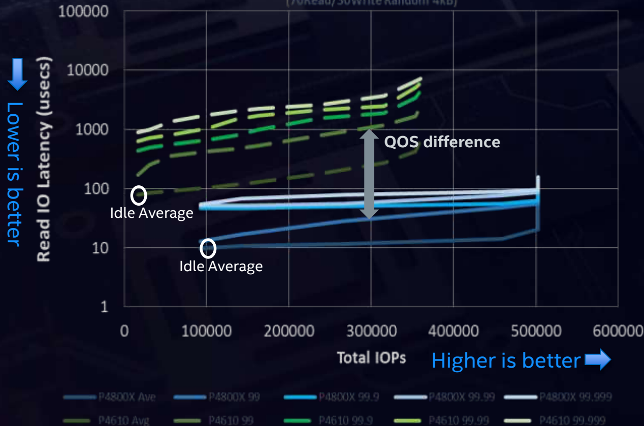
Latency vs. Load: NAND SSD vs. Intel® Optane™ SSD 2 (Intel® DC P4610 3.2TB vs. Intel® Optane™ SSD DC P4800x 375GB) (70Read/30Write Random 4kB)
